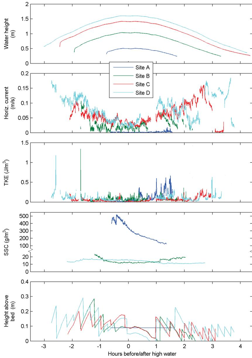
Fig. 4. Time-series of experiment 2 with water level, mean horizontal velocity, turbulent kinetic energy, suspended sediment concentration and the height of the ADV sampling volume above bed. SSC was not measured at location C
