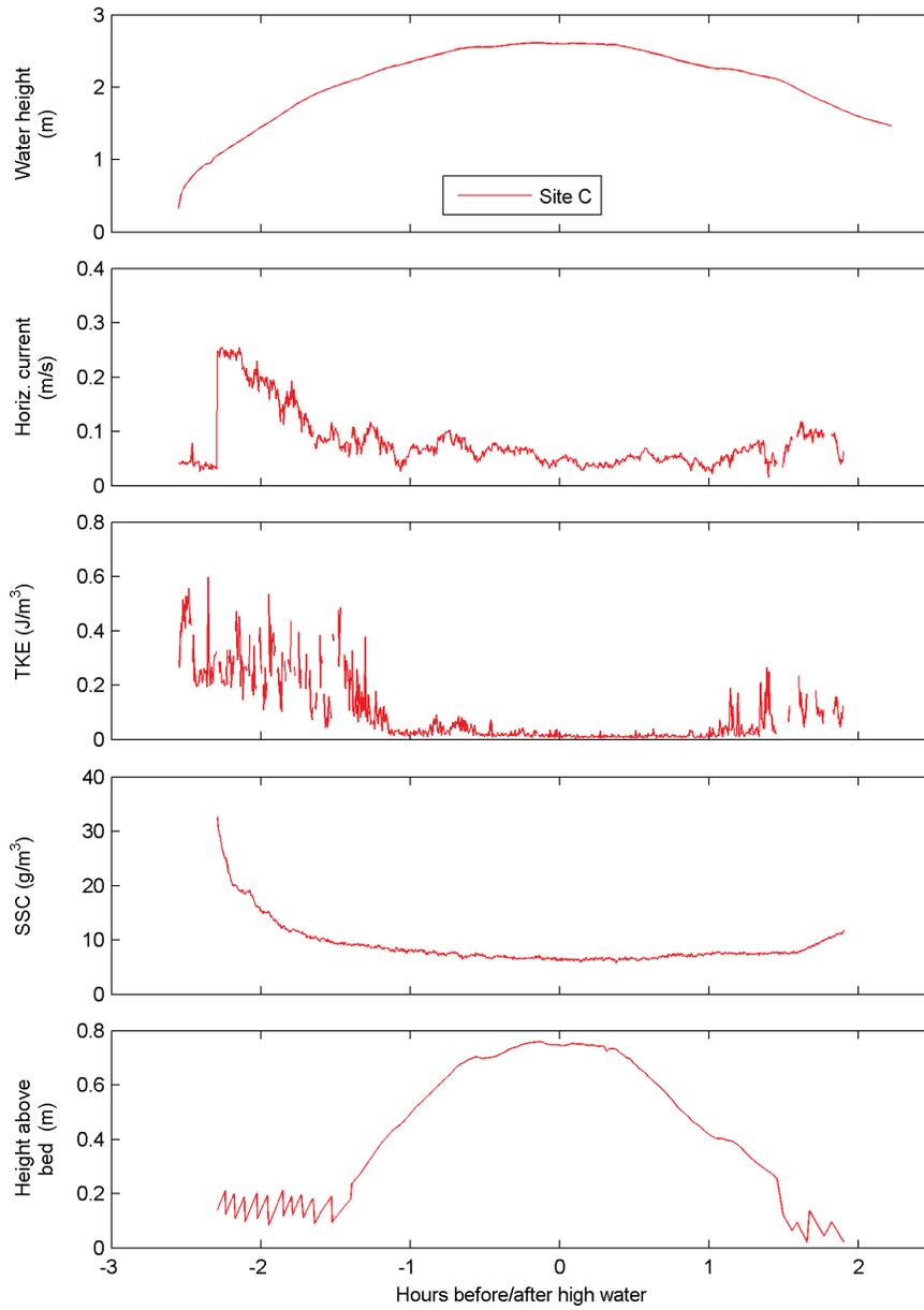
Fig. 3. Time-series of experiment 1 with water level, mean horizontal velocity, turbulent kinetic energy, suspended sediment concentration and height of the ADV sampling volume above bed
