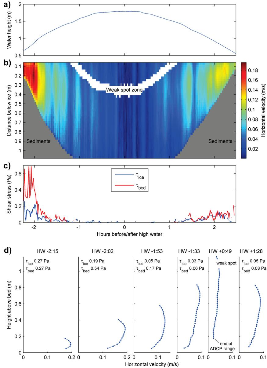
Fig. 6. ADCP results at site B during experiment 3. a) Water level measured with the tide gage. b) Horizontal velocity measured by the ADCP looking downward from the ice base; a weak spot zone occurs at about 1 m from the bed, which is blanked out. c) Shear stress at the ice bottom (upper boundary) and at the bed (lower boundary). d) Examples of profiles of horizontal velocity
