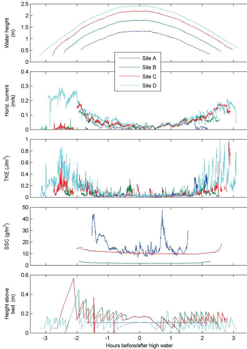
Fig. 5. Time-series of experiment 3 with water level, mean horizontal velocity, turbulent kinetic energy, suspended sediment concentration and height of the ADV sampling volume above bed. SSC was not measured at location D
