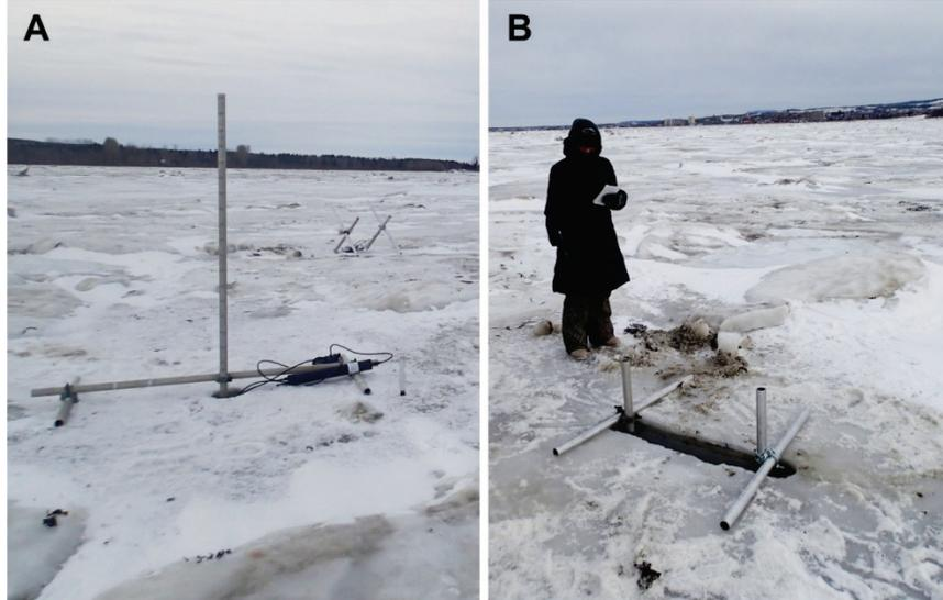
Fig. 2. A) Structure supporting the head of the ADV with the electronic housing on the ice; at the back ADCP with support structure. B) Structure supporting the ADCP
